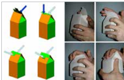
Figure 2. Tuck-in operation by human fingertip and kinematic analysis. From top left to the bottom right: a) first flap folding, b) second flap folding, c) the third flap folding, d) the tuck-in of the third flap.
